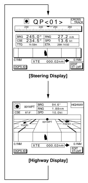
Figure 1-6 Steering display, Highway display
